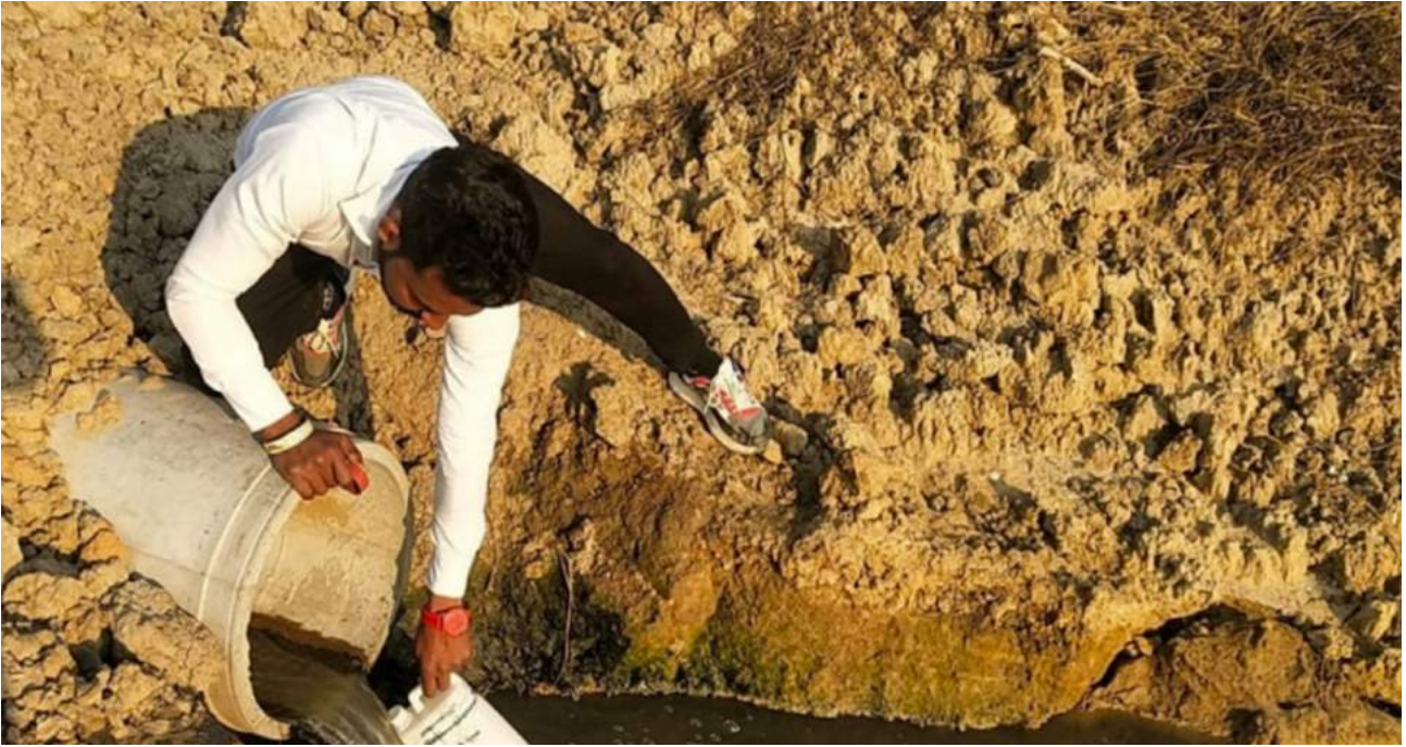
Figure 6: Sample collection from the inlet to the water body where the domestic wastewater is being discharged from.
